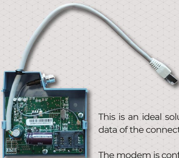
The product's case was designed to fit under the enclosure of the meter and it connects through an RJ45 data connector.
