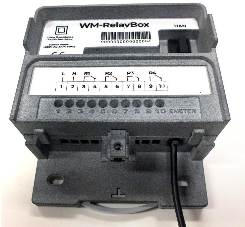
WM-Relaybox with E-Meter connection to a meter device
